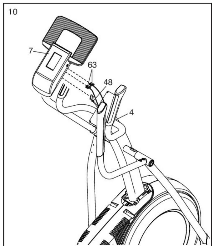
11. **Tip: Avoid pinching the wires.** Attach the Console (7) to the Upright (4) with four M4 x 16mm Screws (101); **start all the Screws, and then tighten them.**
