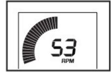
This display will also show the resistance level of the pedals for a few seconds each time the resistance level changes.
