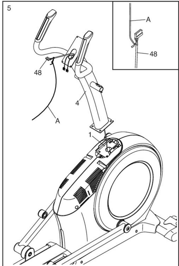
6. **Tip: Avoid pinching the Main Wire (48). Avoid damaging the indicated plastic tabs (B).** Set the Upright (4) on the Frame (1).
