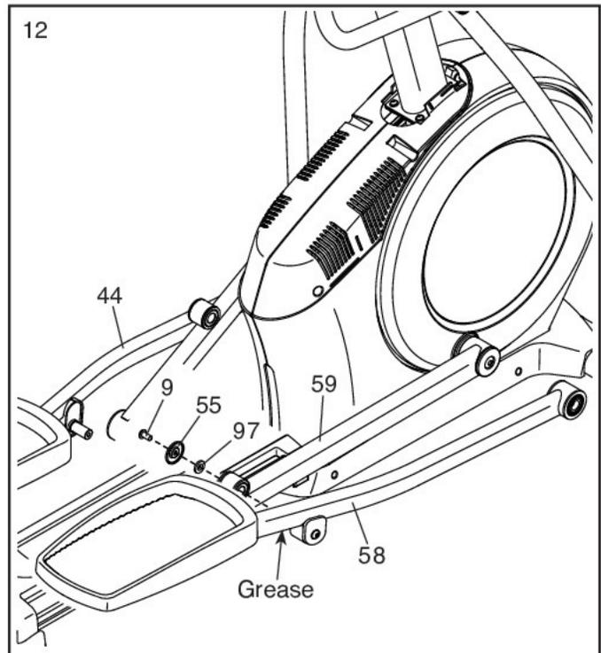
13. Apply a small amount of grease to one of the Pedal Arm Axles (64).
