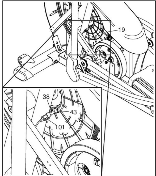
Slightly loosen the indicated M4 x 16mm Screw (101). Slide the Reed Switch (38) slightly closer to or away from the Magnet (43), and then retighten the Screw.
