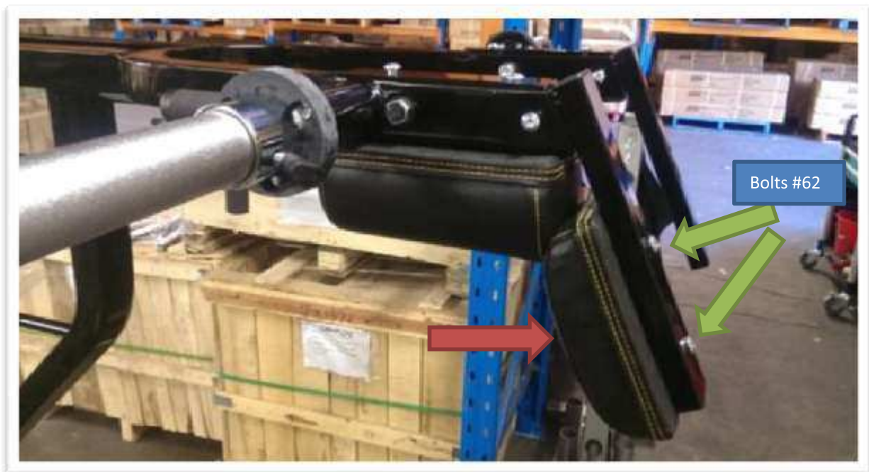
Put the rear support pad on, with bolts #62.
