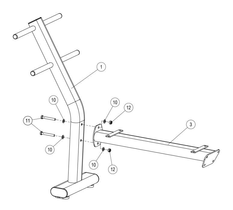
A Attach the Seat Assembly (3) to the Front Support Assembly (1) using 2- M10x70 Hex Screws (11), 4- M10 Flat Washers (10) and 2- M10 Lock Nuts (12).
