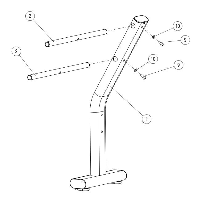
A Attach the Knurled Foot Tube Assembly (2) to the Front Support Assembly (1) using 1- M10x25 Hex Screw (9) and 1- M10 Flat Washer (10).
